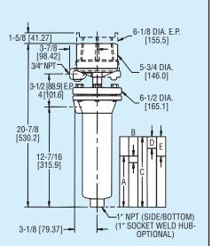
Series 1214 provides vertical connections (1" ANSI forged steel specifications). Flange centerline 15%" mm). Other centerlines available.
