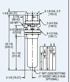
Series 214 has two vertical flanges (1" RF forged steel – ANS specifications). Flange centerline 15%" (403 mm). Other centerlines available.
