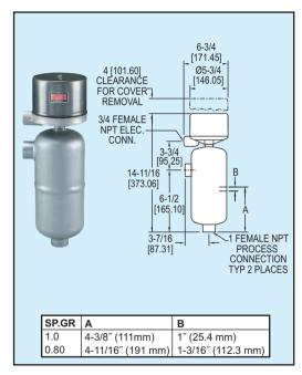
**Heavy duty and low cost** is the perfect description for the 391 Series level control. SS switching mechanism uses gravity return action instead of springs for long life. Weatherproof enclosure is standard. Welded steel chamber is good for 650 psig (45 bar) at 600°F (315°C).
