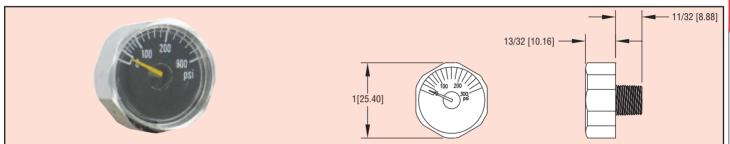
The compact Series SGC2 Pressure Gages are an economical solution for monitoring high pressure applications where space is limited. These 1" gages are perfect for OEM applications for use on pumps, compressors and portable cylinders. The Series SGC2 Gages are housed in a rugged case and feature 1/8" male NPT center back connection.
