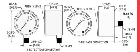
SERIES LPG3 Low Pressure Gages are designed to be especially sensitive with an elastic element that expands and contracts with very small changes in pressure for ASME Grade 1A accuracy. This series is meant for the measurement of low pressures of gases and liquids and is ideal for air flow indicators, liquid level indicators and draft gages. Our new low pressure gages are available in 2-1/2" dial with either a bottom or back connection option.
