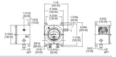
The Series AT22000 ATEX/IECEx Approved Series 2000 Magnehelic® Differential Pressure Gage combines the popular Magnehelic® line with a flameproof enclosure to extend usage to hazardous locations. This gage can indicate positive, negative or differential pressures and is accurate within 2%.
