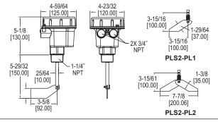
The Series PLS2 Paddle Level Switch is an electromechanical level switch designed for level monitoring of bulk materials. The rotating measuring vane is driven by a brushless synchronous motor at one revolution per minute and as product builds up. the paddle rotation is impeded and the resulting motor torque activates the output switch and stops the motor. The PLS2 is designed with the industry standard 1-1/4" male NPT connection and unit can be side or top mounted.
