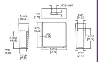
The Model 480 Vaneometer™ Swing Vane Anemometer is a durable, economically priced instrument specifically designed to simplify the measurement of low air velocities. It is accurate to ±5% of full-scale to 100 FPM and ±10% from 100 FPM to the top of scale. It has a spirit level to ensure accurate readings and the large scales are easy to read and visible from both sides.
