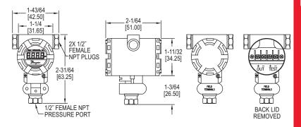
The Series IWP Industrial Weatherproof Pressure Transmitter provides an exceptional value solution to pressure measurement in industrial conditions requiring high-performance, stability and long service life. The precise operation under dirty and wet conditions, make the Series IWP an ideal choice for petroleum, chemical and metallurgical industry applications.
