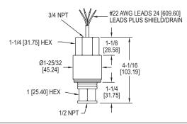
The Series 636 Fixed Range Pressure Transmitter is a low cost, fixed range, stainless steel transmitter with ±0.30% accuracy. It is designed to continuously measure pressure for years in even the toughest environmental and media conditions. Transmitters are explosion-proof, (FM approved) and meet NACE standards for offshore applications.
