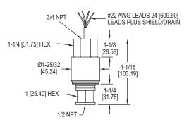
The Series 636 Fixed Range Pressure Transmitter is a low cost, fixed range, stainless steel transmitter with ±0.30% accuracy. It is designed to continuously measure pressure for years in even the toughest environmental and media conditions. Transmitters are explosion-proof, (FM approved) and meet NACE standards for offshore applications.
