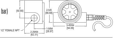
The Series SF Sight Flow Transmitter is a Series of sight indicators which can display flow or contents of pipelines and provide an analog 4-20 mA signal proportional to the flow rate. It is available with a 316 SS or clear polycarbonate cover.
