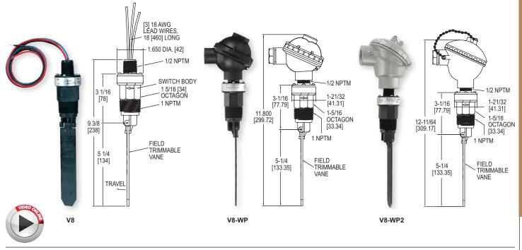
The Series V8 Flotect<sup>®</sup> Vane Operated Flow Switches are ideal for protecting unattended equipment from damage or loss of production. This Series is available for installation in a 1 to 6" pipe with operating pressures are up to 150 psig (10 bar) and temperatures to  $212^{\circ}$ F ( $100^{\circ}$ C).
