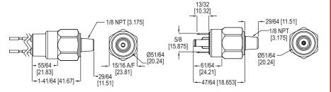
Designed for OEM applications, the Series A2 Subminiature Pressure Switch is economical and is equipped with high proof pressure capabilities for demanding applications. The A2 is available with either spade terminals or flying leads (submersible). Switches with spade terminals can be easily adjusted in the field.
