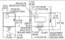
Reliable and convenient, the Series AP Diaphragm Operated Pressure Switch is a compact switch for instrument air or other low pressure applications. Visible set point and external adjustment add convenience. Used on air, non-corrosive gas or liquid service compatible with wetted parts. Units are available in weather-proof and explosion-proof housing.
