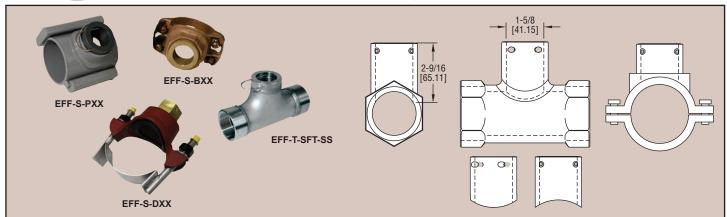
The Series EFF Fittings and Tees are used with the Series EFS2 Insertion Electromagnetic Flow Sensors. The Series EFF allows for sensor insertion in a wide range of pipe sizes. Multiple end connections are available to allow for easy installation in many applications. Series EFF is available in bronze, 304 stainless steel, 316 stainless steel, and PVC, further expanding application prospects.
