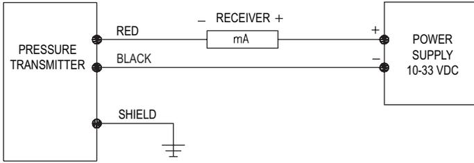
The maximum loop resistance (RLmax) for the DC power supply voltage (Vsup) is expressed by the formula:
