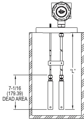
Figure 1: Attached Ground Rod Option
