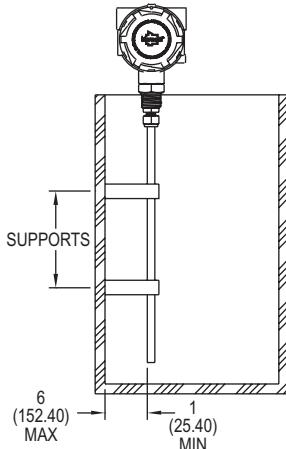
Figure 2: Supports to Tank Side Wall
