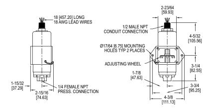
Series 1000E explosion-proof also available in 1000EH explosion-proof, hermetically sealed switch assembly.
