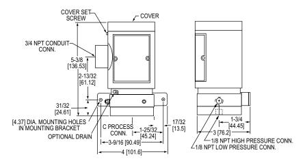
Series H3 Differential Pressure Switches actuate one or two single pole, double throw (SPDT) snap switches in response to increasing or decreasing pressure of compatible gases or liquids. Four field adjustable operating ranges are available allowing set-points up to 200 psid. All models are suitable for hazardous locations and also include weatherproof housings as detailed in the chart below. Read and understand instructions completely before proceeding with installation or operation.
